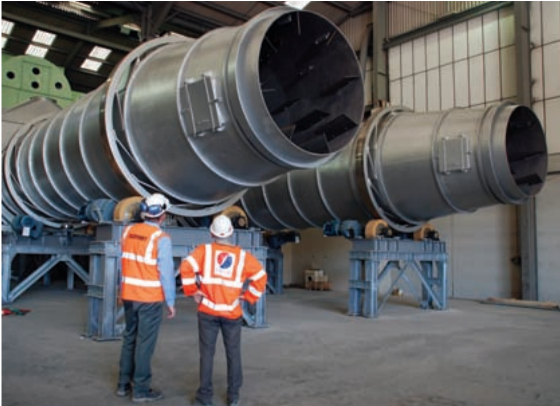
The Demonstrator's unique waste-processing drums being fitted on site.
